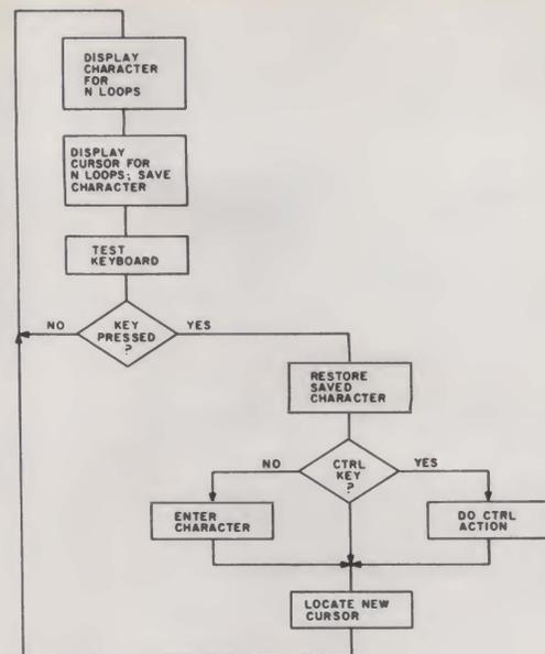
Fig. 8. Flowchart for an editing display that combines a winking software cursor within the keyboard testing loop.
